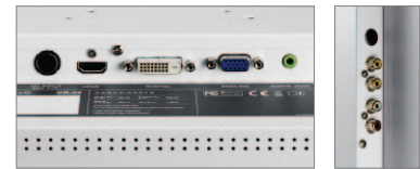
Analogue, DVI, S-Video, CVBS and HDMI inputs for video device or PC data feeds
